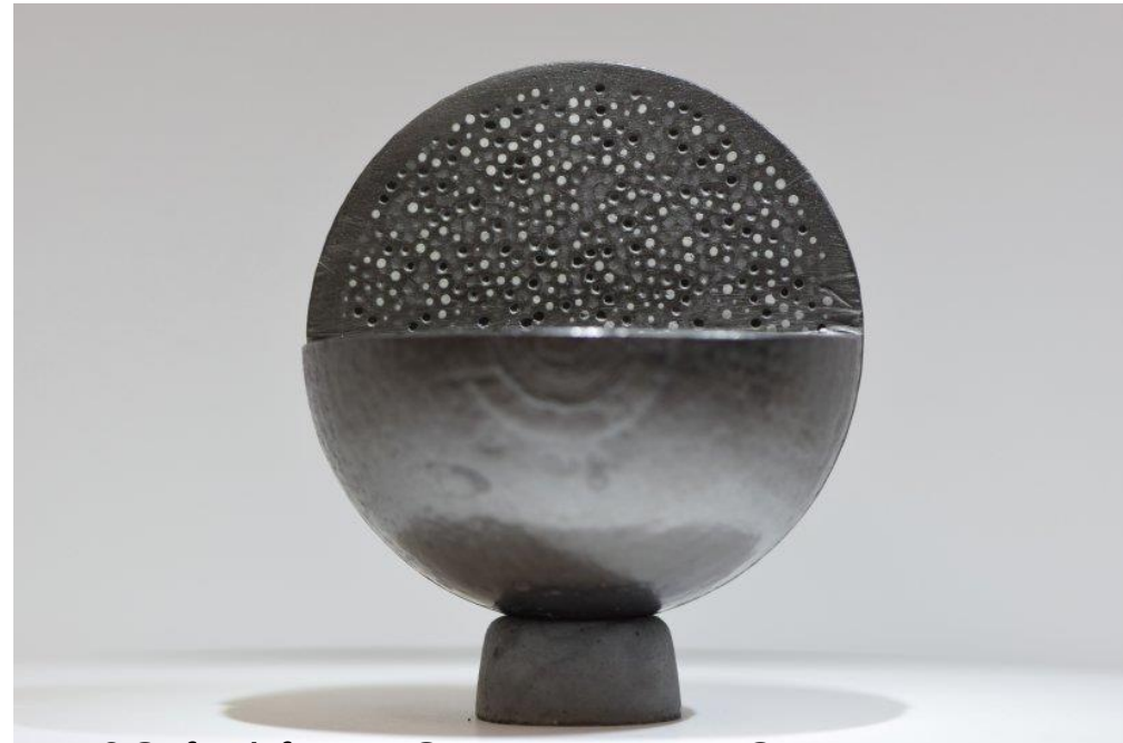
TRISO fuel for HTGRs, courtesy DOE.
